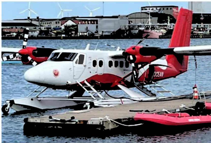
Figure 21: Nordic Seaplane docked at Langelinie, fueling over the water with no visible drip-prevention system. Photo Credits: Thomas Gray, May 2025
