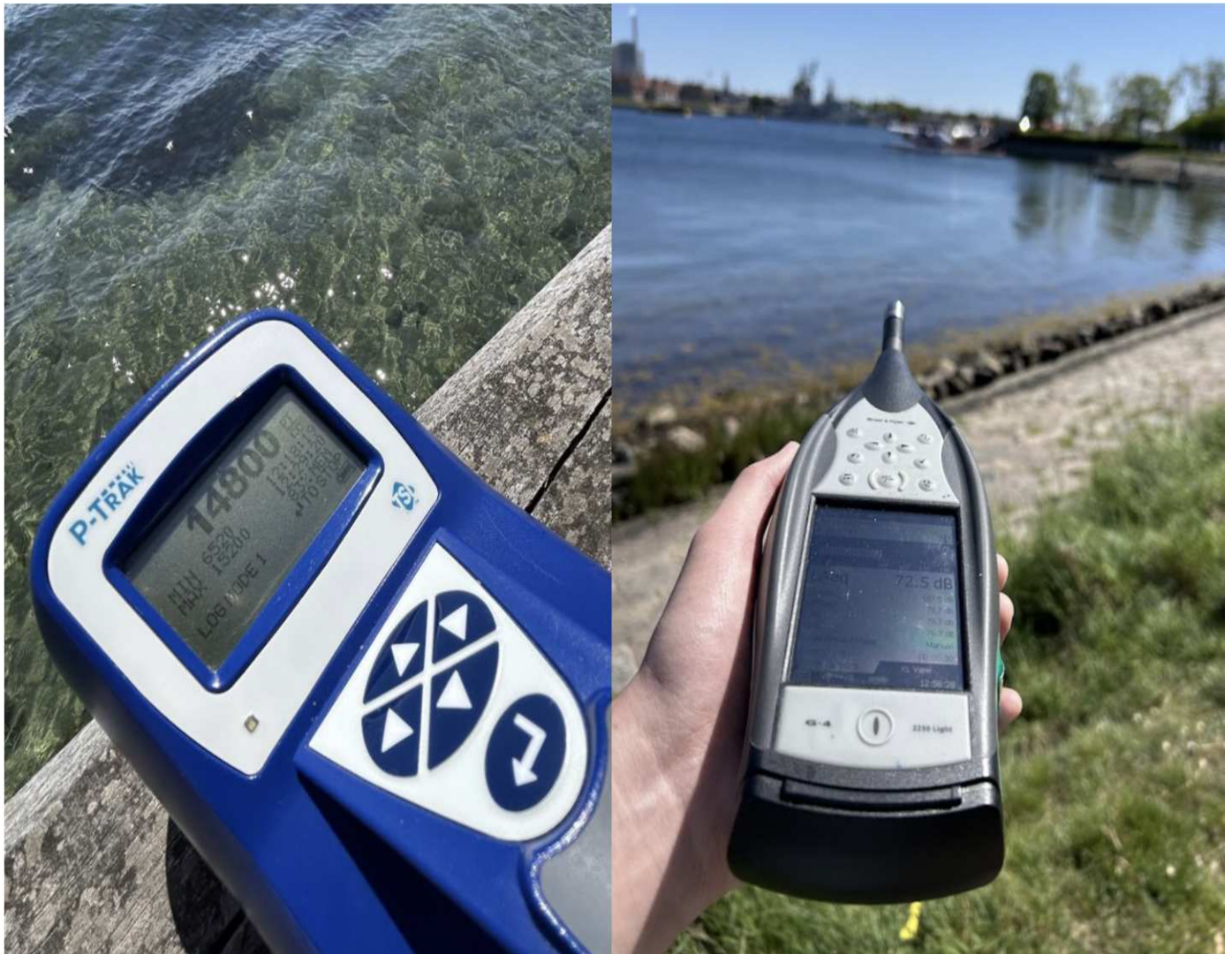
Figure 13: P-Trak 8525 Ultrafine Particle Counter (left) and the Brüel & Kjær 2250 Sound Level Meter (right) being used near Langelinie Park. Photo Credits: Dante Nguyen
