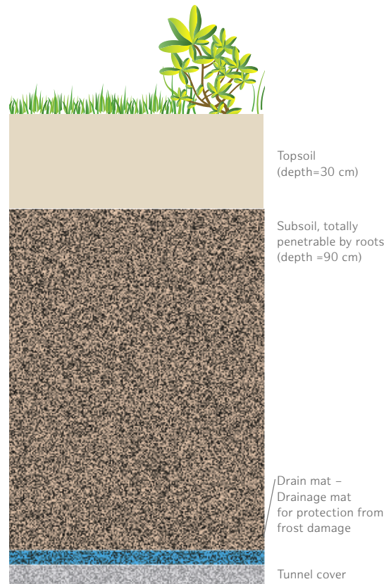
Schematic representation of the soil structure on the 'Hamburg Roofs'
