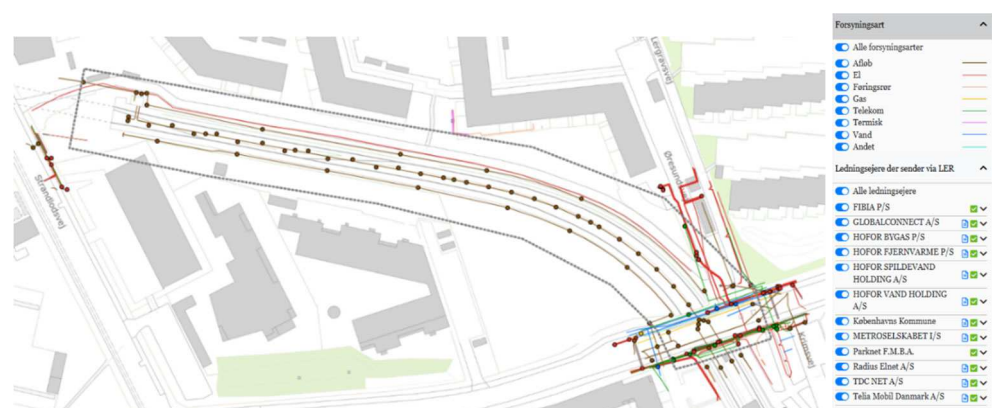
Figure 5: Cables and utilities around the trough
