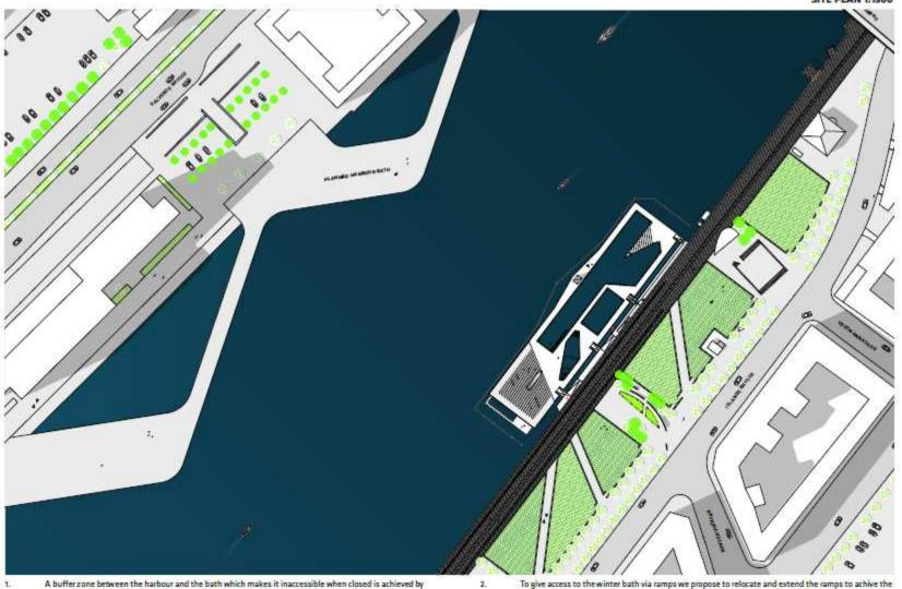
1. A buffer zone between the harbour and the bath which makes it inaccessible when closed is achieved by shortening the access stair and ramps. A most between the bath and the access area is created.
