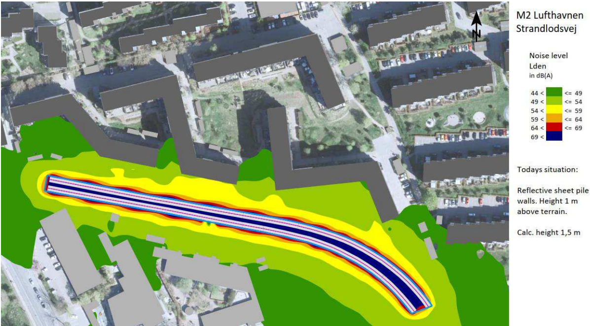
Figure 8 – Current situation. Noise propagation at ground-level height (1.5 m)
