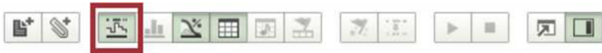
Figure 26: Graph display button located in the top right of the BZ-5503 Measurement Partner Suite.
