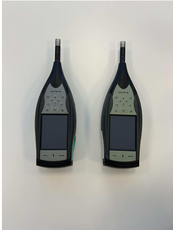
Figure 9: Hand-Held Analyzer Type 2250 Light [LEFT] and Type 2250 [RIGHT] from Brüel & Kjær.
