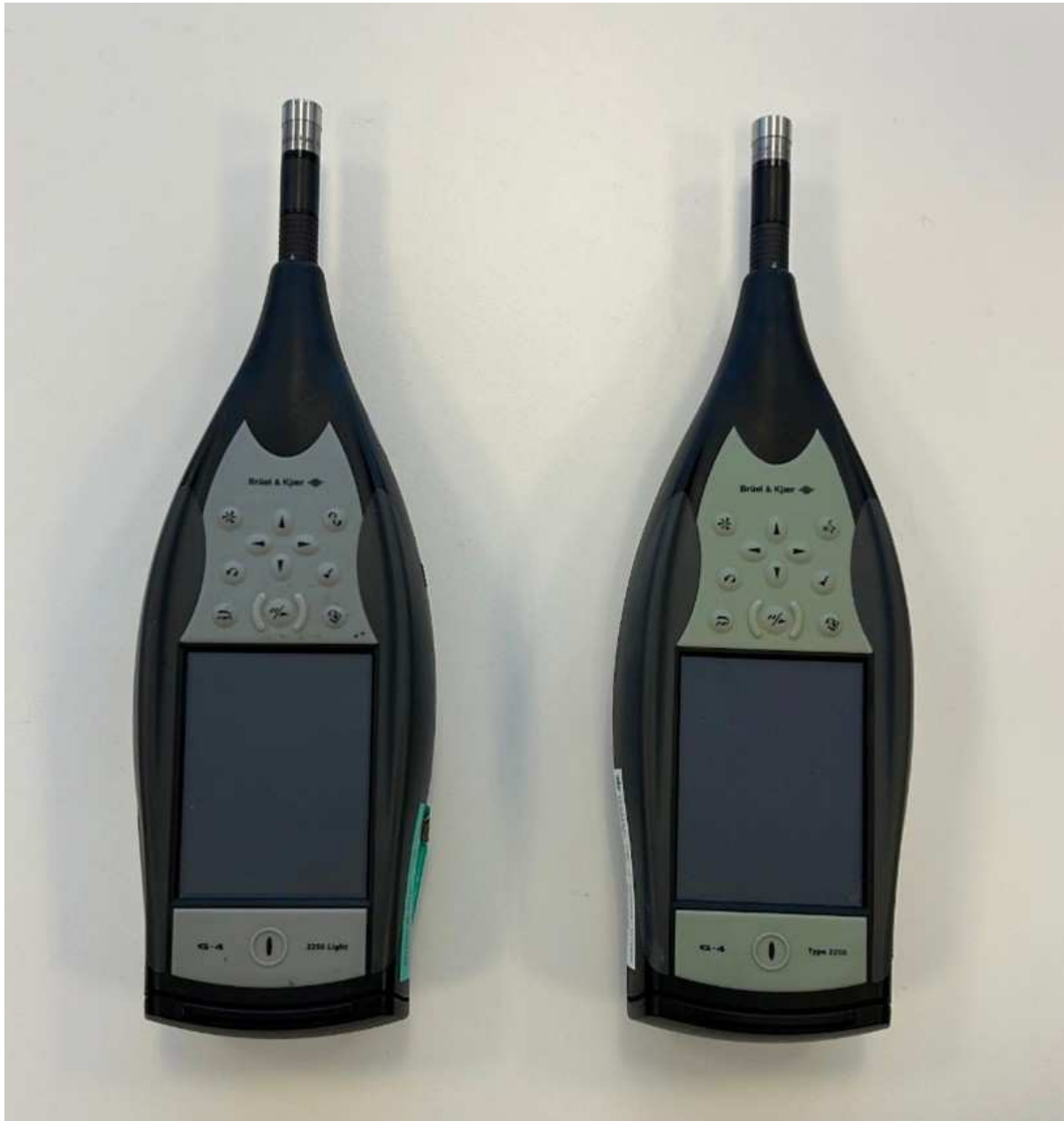
Figure 25: Brüel & Kjær Hand-Held Analyzer Type 2250 Light [LEFT] and Type 2250 [RIGHT].
