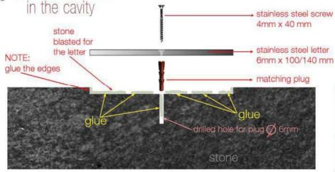
The glue should be Rotabond, soft polymerglue
