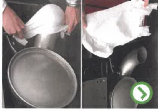
Figure 13: Steps of the Handkerchief test 6
